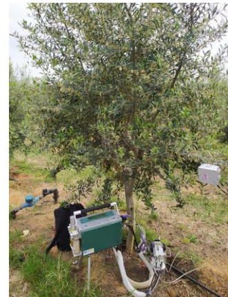
Open gas exchange system (LI-6400, Li-Cor)
