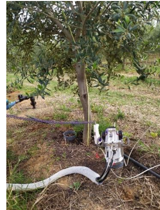
Open gas exchange system (LI-6400, Li-Cor)
